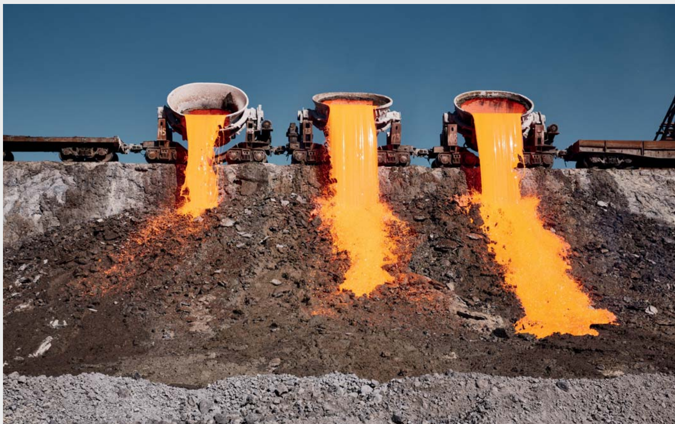
Lime is required for slagging in ironmaking.
