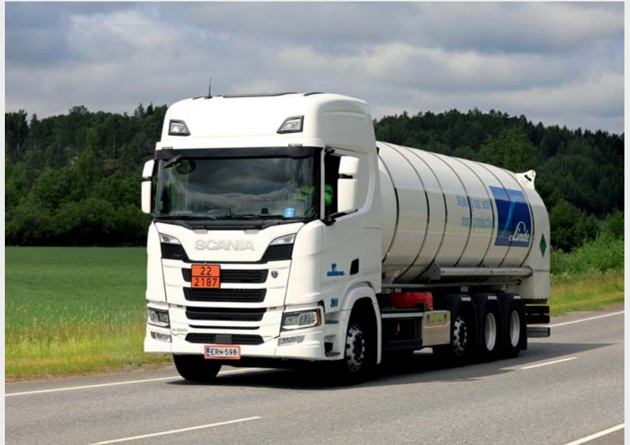
Cryogenic liquid \text{CO}_2 distribution by road
