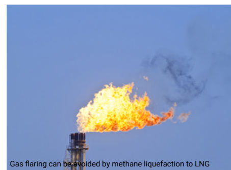
Gas flaring can be avoided by methane liquefaction to LNG
