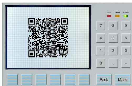
Figure 3 QR code displayed on a gas analyser control panel for communication of diagnostic information via a smartphone or tablet Photo: ABB
