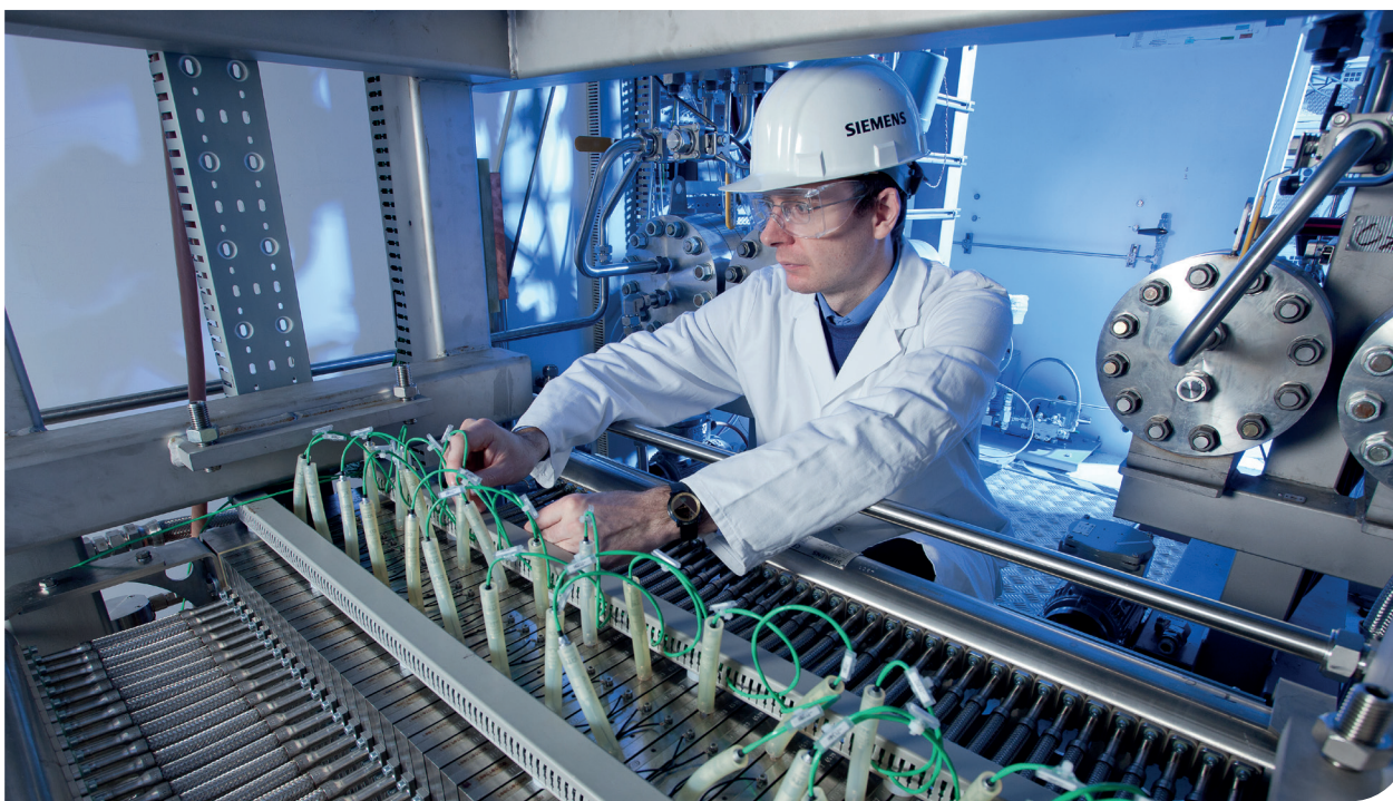
Silyzer electrolyser for hydrogen production, Copyright Siemens Energy
