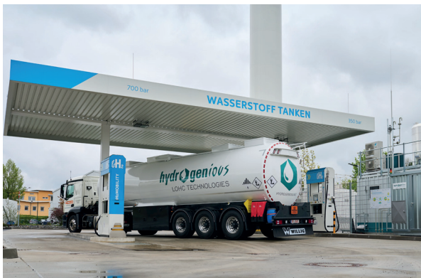
Hydrogenious benzyltoluol LOHC supplied to the HRS Erlangen, Copyright HyPlus
