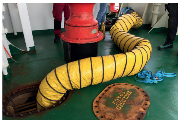
Forced ventilation of a confined space on board ship prior to entry
