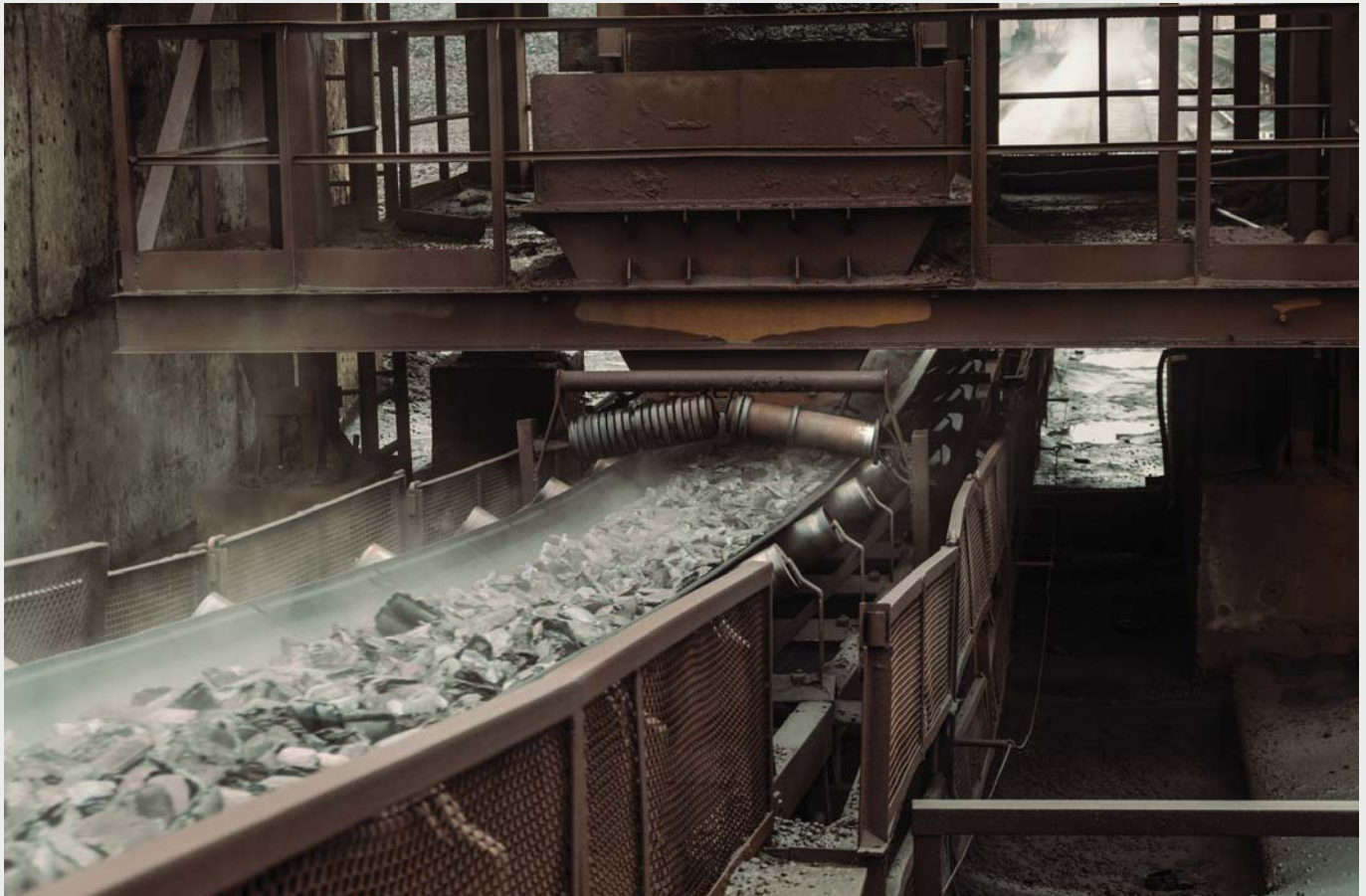
DRI and HBI have porous structures, which makes them prone to re-oxidation in contact with air or moisture. This causes self-heating.
