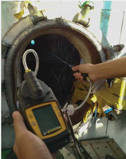
Bulk cargo such as DRI presents spontaneous combustion hazards that must be monitored using gas detection equipment.
