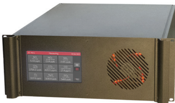
Copyright MIRO, 10 component QCL gas analyzer
