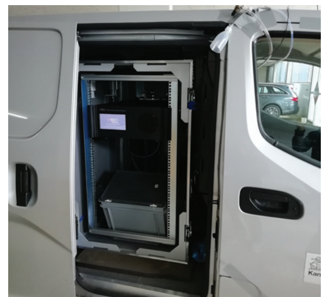
Copyright Michael Götsch, AWEL - MIRO QCL gas analyser used for the Gubrist Tunnel test
