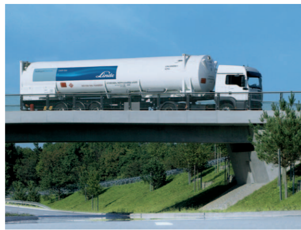
Figure 4. When smaller quantities of hydrogen are required, it can be supplied by tube trailer, stored on site in liquefied format and then vaporised for use as gaseous hydrogen.
