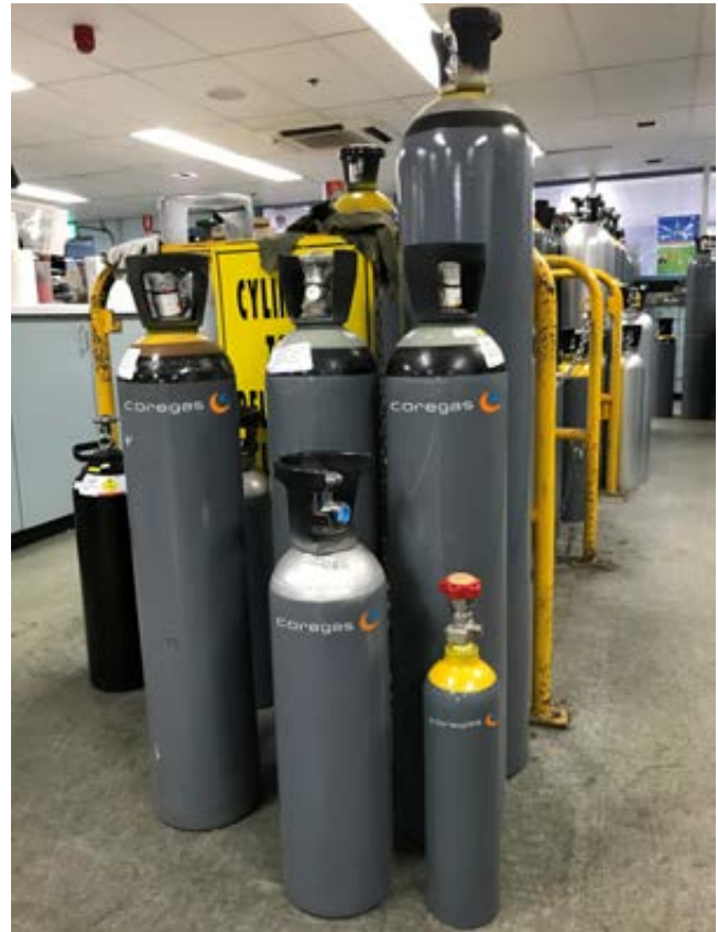
Coregas specialty gas mixture cylinders for gas detector bump testing and calibration
