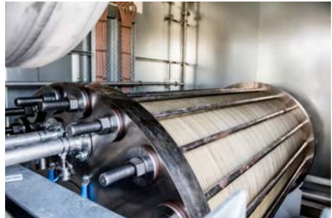
0.5 MW, 200 cubic metres per hour McPhy Hydrogen Electrolyser. Copyright RAG & Karin Lohberger Photography.
