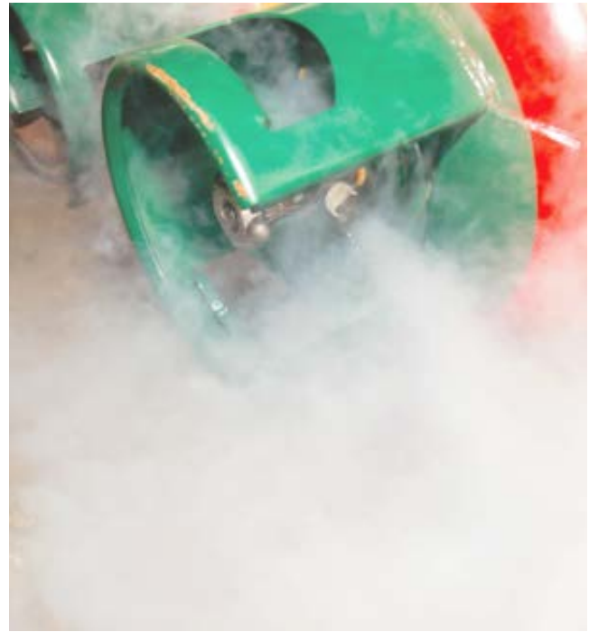
Leaking ammonia gas cylinder
