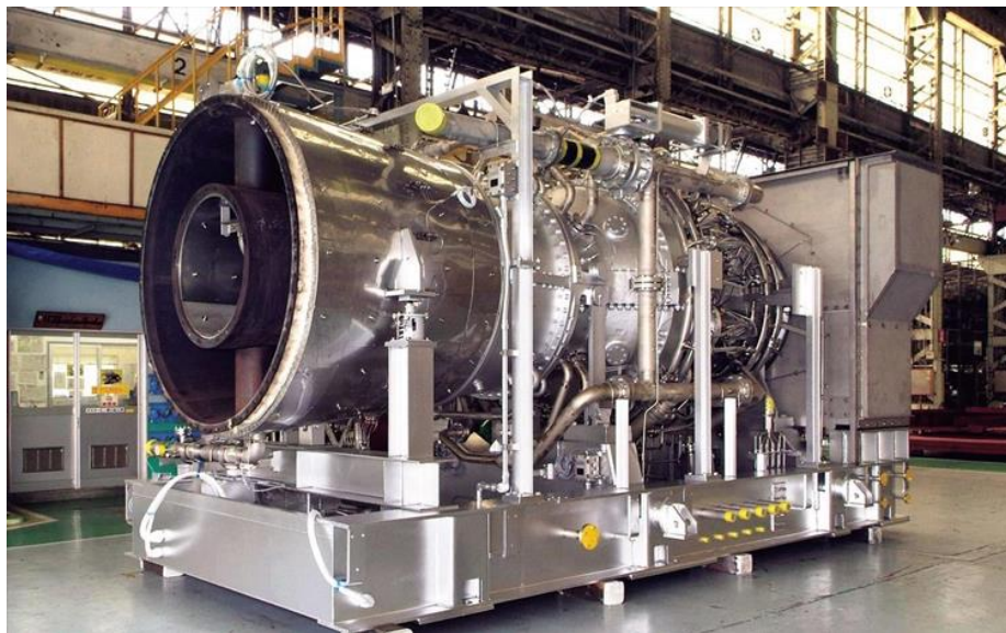
Mitsubishi Power H-25 Series gas turbine, 40MW class
