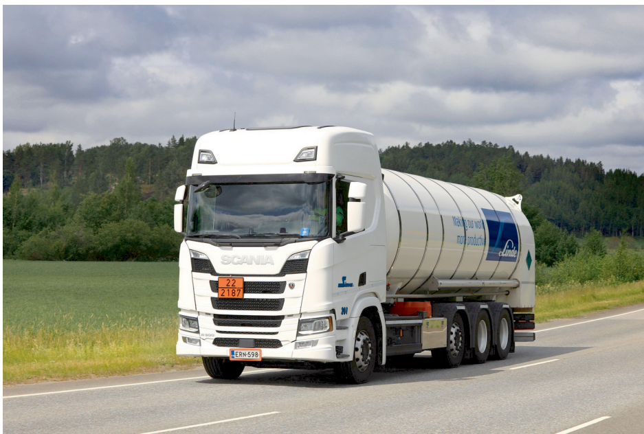
Cryogenic CO 2 distribution by road
